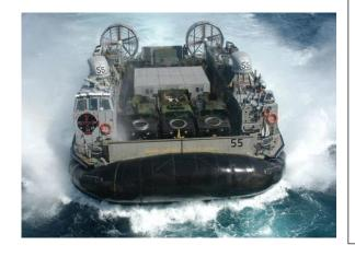
Newton's first law states that an object in motion will stay in motion unless an external force acts upon it. One common opposing force is friction. A hovercraft uses blowers to produce a large volume of air beneath it, producing lift, reducing friction, and allowing it to glide over land, water, mud, or ice. Following the directions below you can build your very own model hovercraft!
