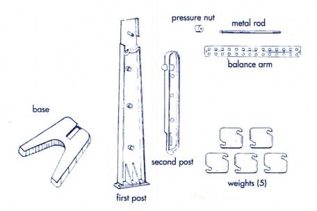
To assemble, slide the first post into the base. Attach the second post to the first post and fasten with the pressure nut. Push the metal rod into the hole at the top of the second post. Turn the balance arm so that the side with the holes numbered from the center in both directions faces you. Slide the top unnumbered center hole onto the metal rod. If the arm doesn't balance, put small bits of clay on the lighter side until it does balance.
