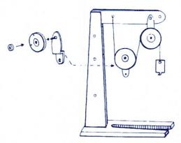
Why do you think this second pulley is called a "moveable pulley"? If you hang one weight from the moveable pulley, how many weights must you hang on the end of the string to balance it? Hang two weights on the moveable pulley. How many weights must you hang on the end of the string to balance these? Hang four weights on the moveable pulley and determine the number to be hung on the string.
