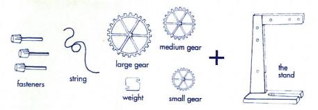
Before you assemble the parts, use a magic marker or a tiny piece of colored tape to make a dot on one tooth of each of the three gears. This will make it easier for you to count the number of times each gear turns during the explorations.
