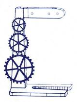
Turn the gears so all the dots are at the top. Turn the large gear around once. How many times did the small gear turn? Did it turn faster or slower than the large gear?
