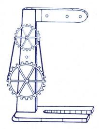
Fasten the rubber band so it crosses itself between the gears as shown in the sketch.
