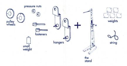
Move the second post of the stand so that is is horizontal. Attach one pulley to a hanger with a pressure nut. Push the hanger into the middle hole of the stand as shown.
