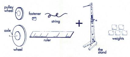
Remove the balance arm and weights from the stand you assembled before. Attach the wheel and axle assembly to the stand using the fastener as shown.
